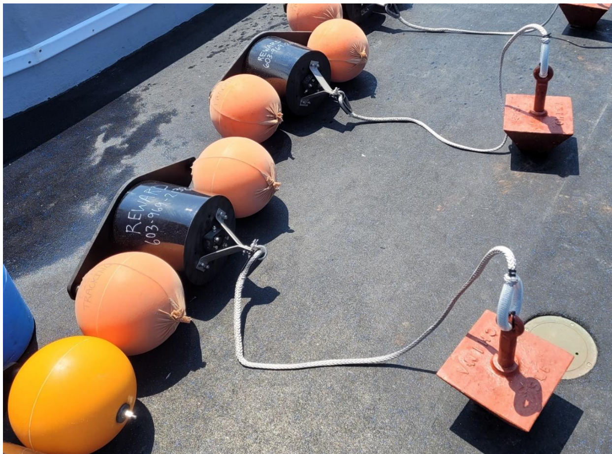
Figure 2 – Recoverable and reusable mooring configurations used to deploy VEMCO VR2AR acoustic receivers.
