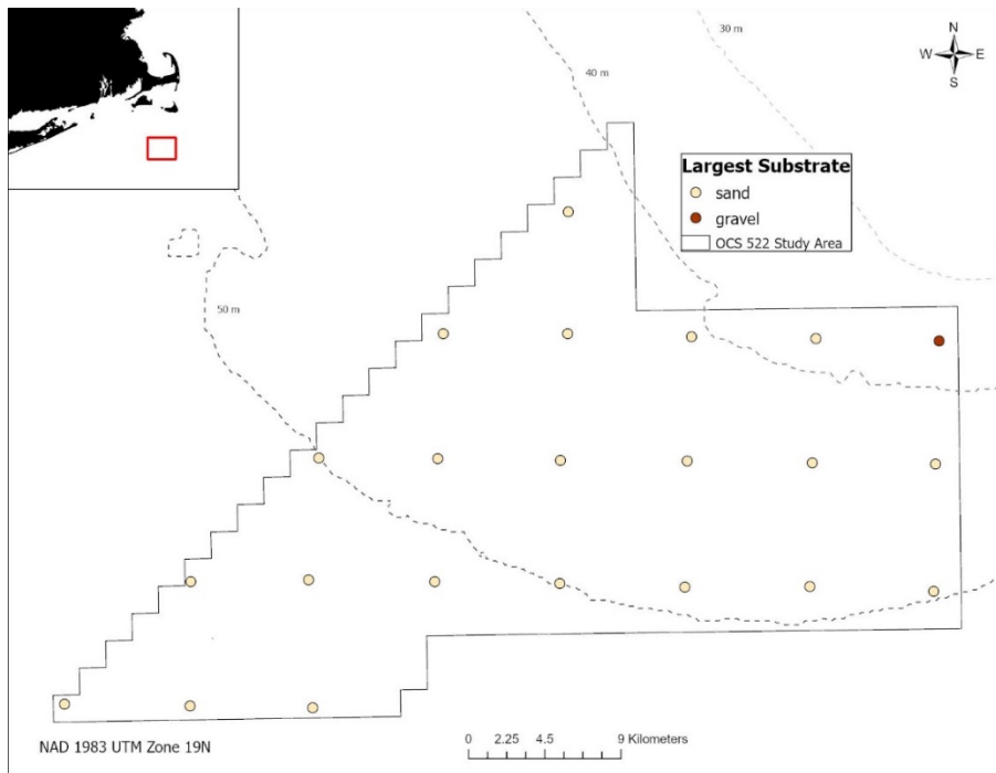
Figure 25. The distribution of the largest observed substrate type from the May 2022 drop camera survey of the 522 Study Area. Four quadrats (2.3 m 2 images) were observed at each station. Note, more comprehensive efforts have been completed by Vineyard Offshore to classify the benthic habitat in Lease Area OCS-A 0522 and are reported elsewhere.
