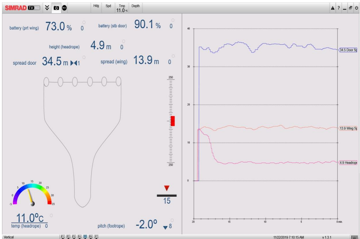
Figure 7: Screenshot of the SIMRAD TV80 software monitoring the trawl parameters.
